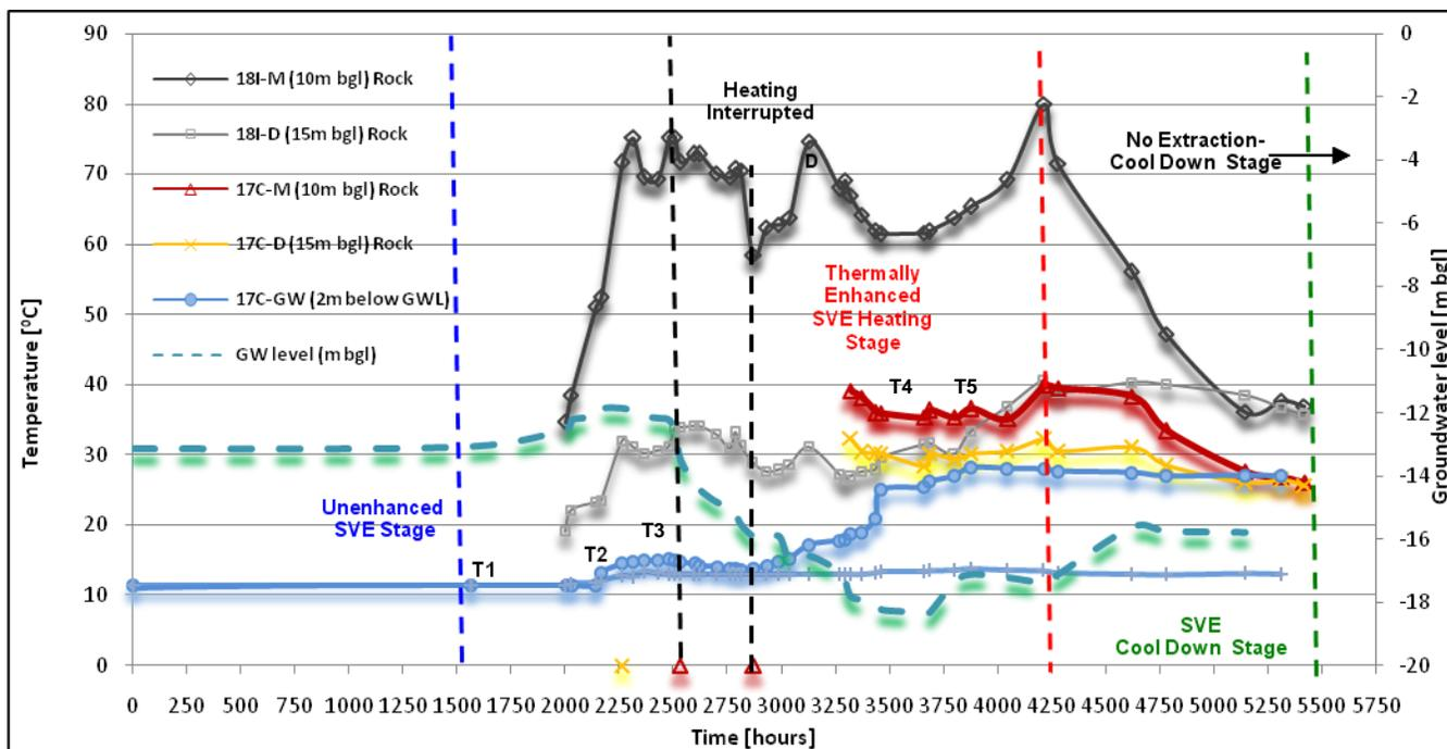
**Figure 6: Rock mass temperature, groundwater levels and temperature profile against time during remediation process at Pit No.18**
