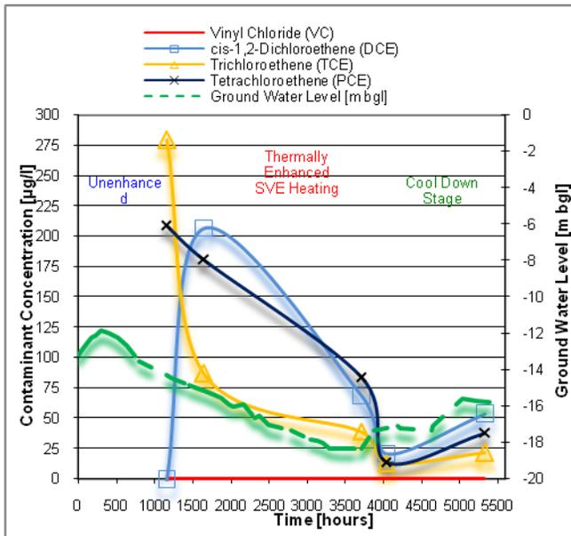
Figure 7: Groundwater chlorinated ethenes concentration trend for well 17B (located within TTZ).
