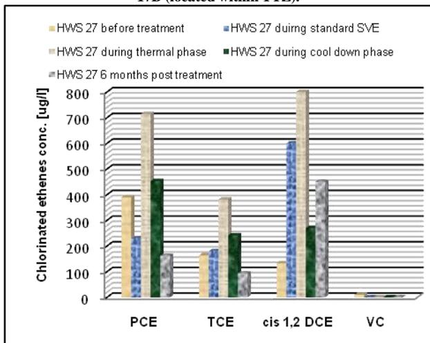
Figure 8: Groundwater chlorinated ethenes concentration trend for well HWS27, before during and following thermal remediation at Pit No.18.
